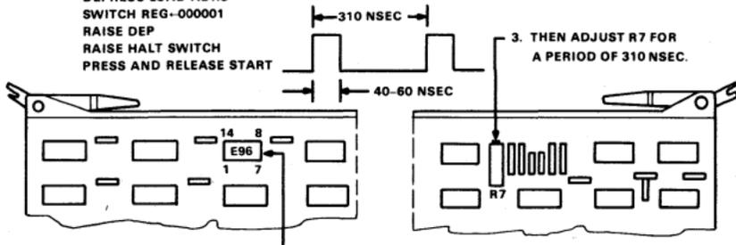
2. PLACE SCOPE PROBE ON E96 PIN 9
