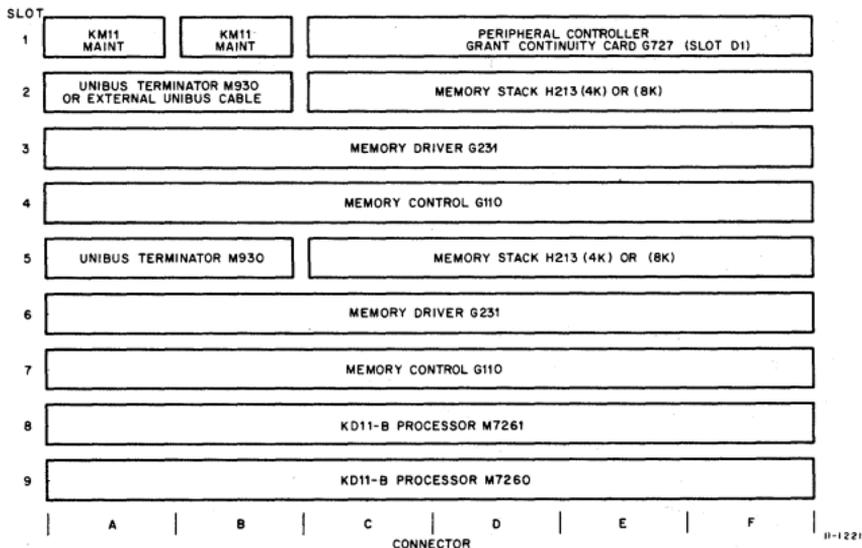
**PDP-11/05-LA MODULE UTILIZATION (8K)**
