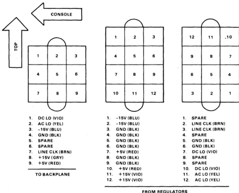
In the mainframe box's distribution panel, there are three groups each containing five connectors, that is, the two 12-pin connectors shown above and three of the 9-pin connectors shown above. Within a group, all three 9-pin connectors are bussed together pin-for-pin by the distribution panel. Each connector may or may not have all the above-listed wires connected to it.
