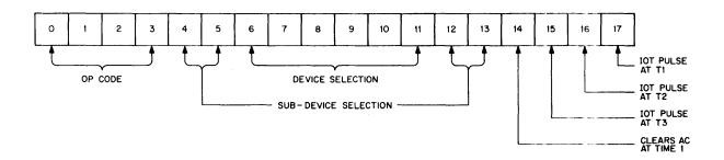
The following table indicates the bit assignments (in octal) used to program the 340 Display.
