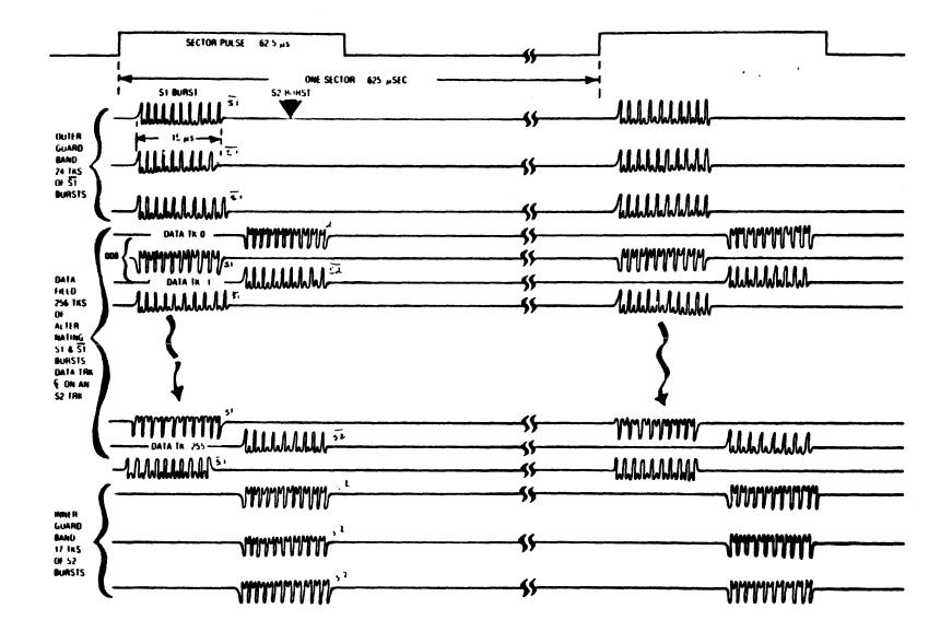
Figure 1 RL01 Servo Data Format
