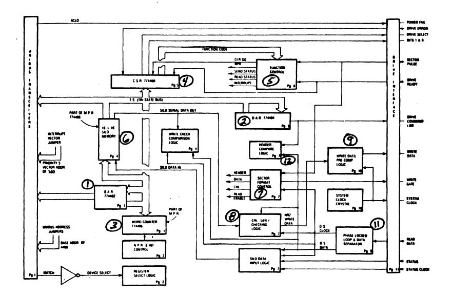
Figure 6 M7762 RL11 Basic Block Diagram
