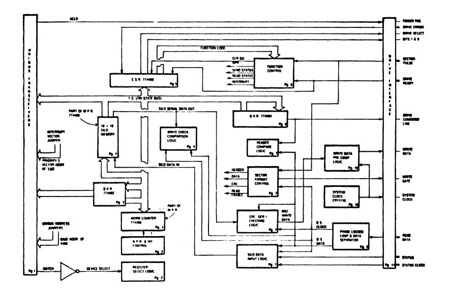
Figure 2 M7762 RL11 Basic Block Diagram
