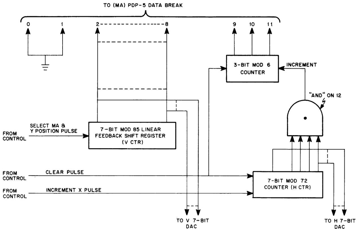
Figure 2 Memory Address and X-Y Position Logic
