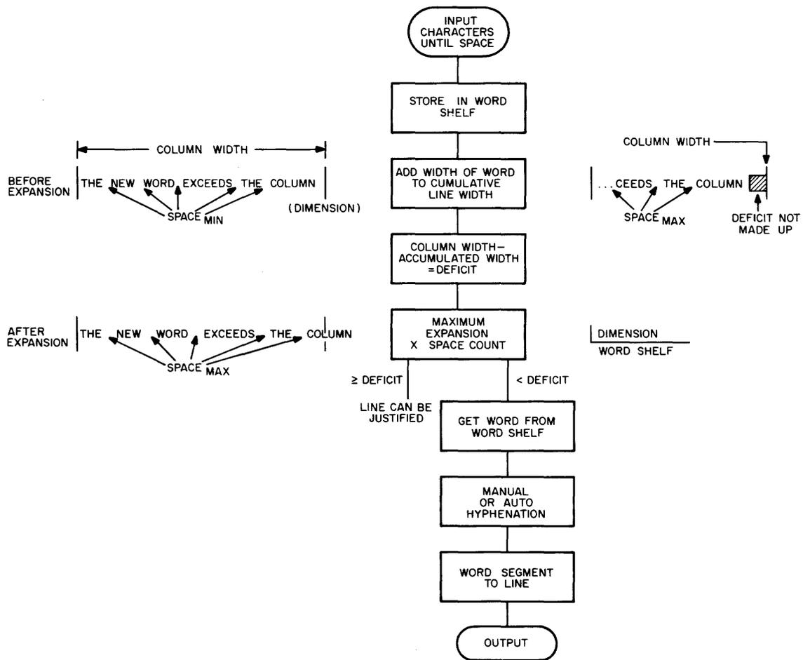
Figure 9 Justification-Hyphenation Schematic
