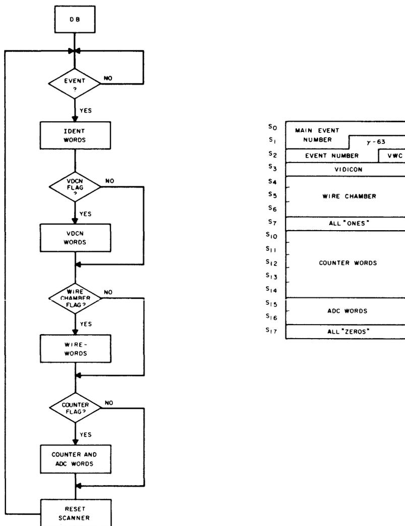
Figure 6 Data Source Control Scanning Procedures
