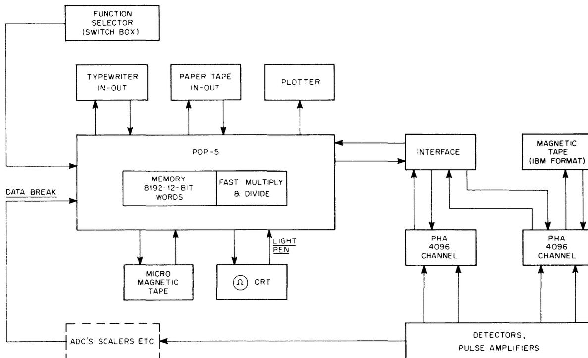
Figure 1 Block Diagram PDP-5 88" Cyclotron System
