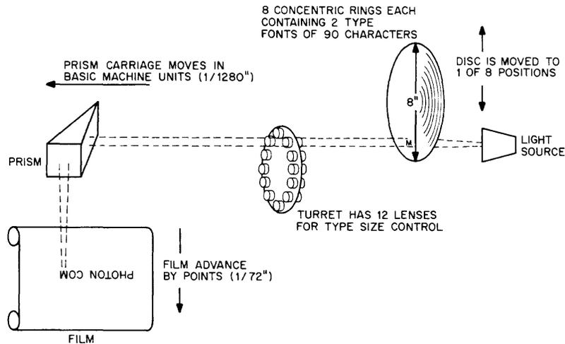
Figure 7 The Optical System of the Photon
