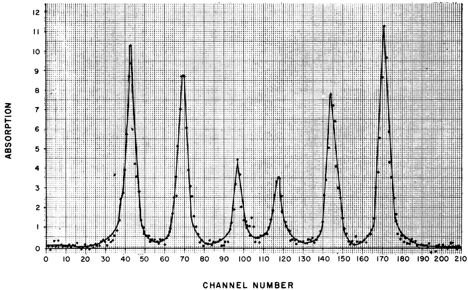
Figure 9 Mossbauer Spectrum of Iron Metal
