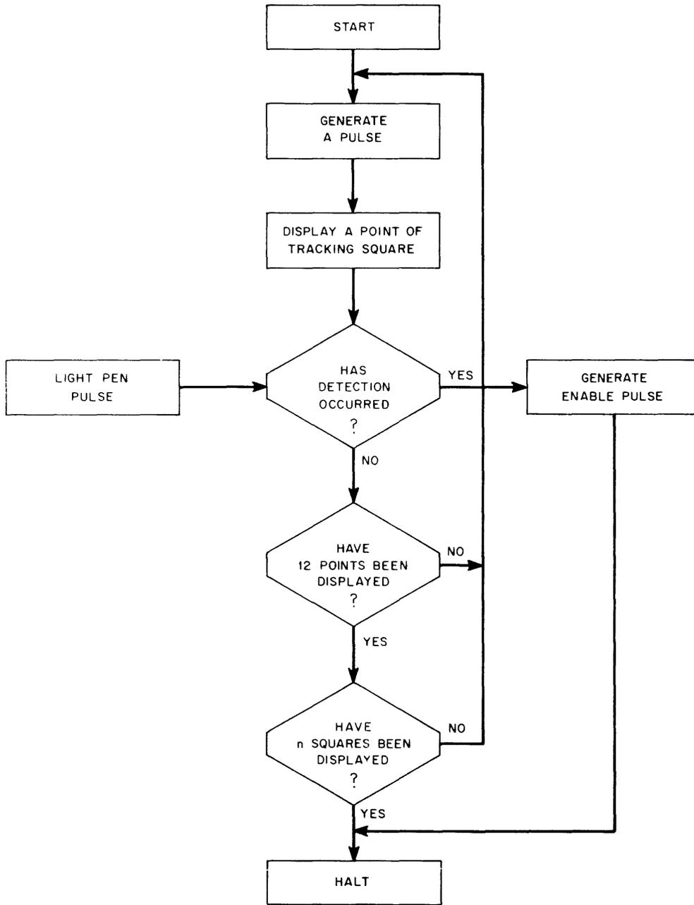
Figure 7 Flow Diagram Light Pen Tracking Unit
