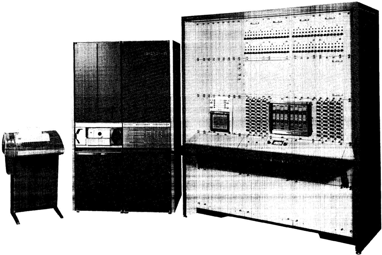
Figure 3 AD-80 and PDP-5 Hybrid Computer System
