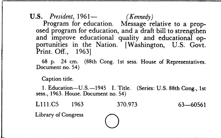
Copy of Library of Congress style catalog card typeset automatically from the input perforated tape record. The tape produced from typing the recording form was processed by a digital computer, producing a second tape which controlled the phototypesetting machine. The output of the phototypesetting machine is the card shown.
