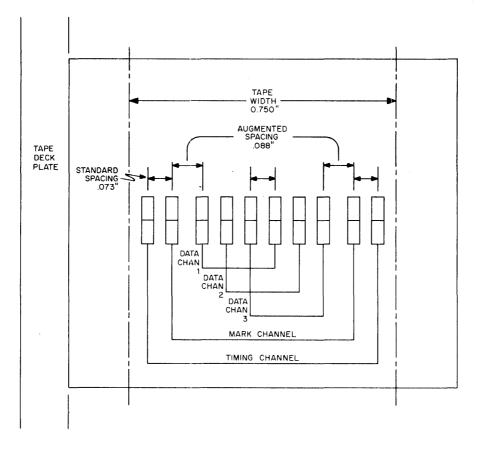
Figure 1-3 Arrangement of DECtape Head
