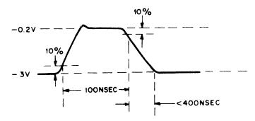
Figure 5-2 FLIP CHIP R-Series Pulse
