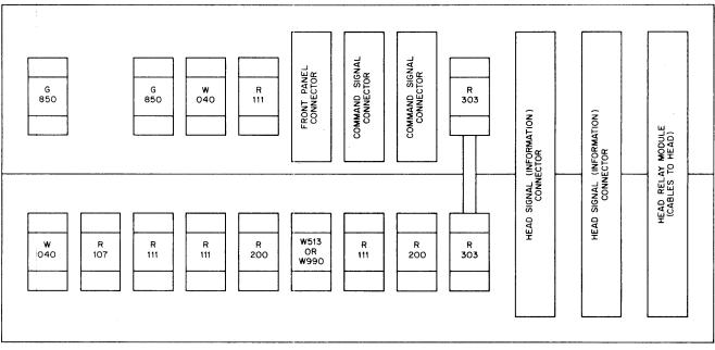
Figure 1-5 TU55 Interface Connections
