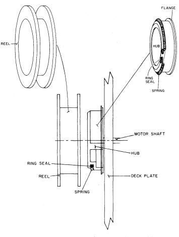
Figure 1-2 Hub and Reel Assembly
