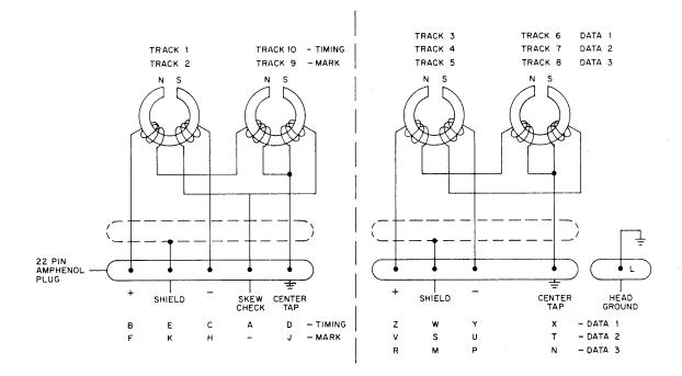
Figure 2-2 Head Connections
