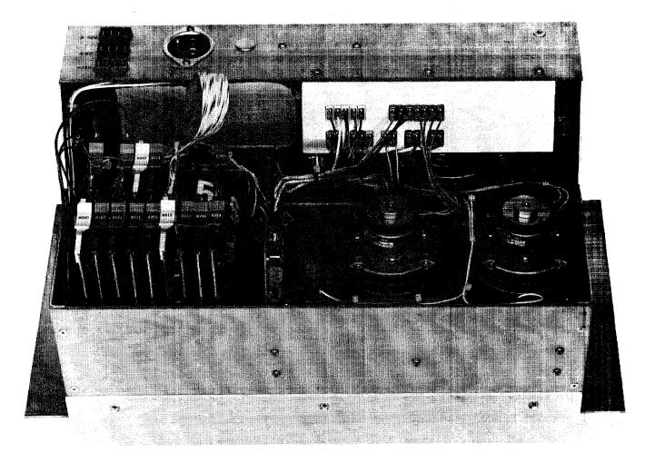
Figure 1-4 Type TU55 DECtape Transport, Rear View
