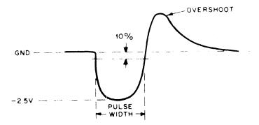
Figure 5-3 FLIP CHIP B-Series Pulse
