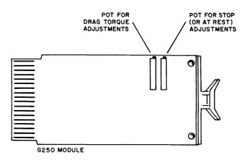
Figure 4-1 Module Adjustment Trimpots
