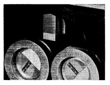
DECtape transport showing the two 3<sup>1</sup>/<sub>2</sub>-inch reels and their relationship to the tape guide and the read-record head assembly.
