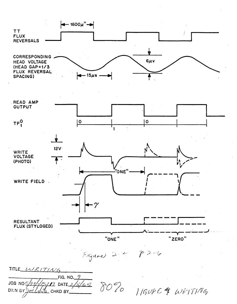
of approximately 33 µsec; at the end of this time, the next TP1 pulse shifts the register to create (possibly) a new pattern. Accordingly, the AND circuit outputs can be asserted only for 33 µsec. Thus, after the mark track heads read into the window register a particular pattern as created by the last bit read, the AND circuits, fed by the register, are allotted a time interval of 33 µsec in which to recognize the pattern and produce the appropriate responses.
