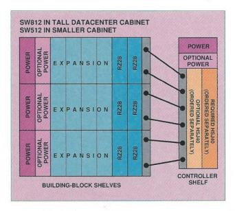
building block is a 5.25-inch disk drive mounted in a carrier that occupies three slots in a building-block shelf. Each shelf is cabled to a separate port on the HSJ40 controller. The six building-block shelves, plus a controller shelf, are installed in the SW800 cabinet to make the SW811 subsystem, or in the SW500 cabinet to make the SW511 subsystem.
