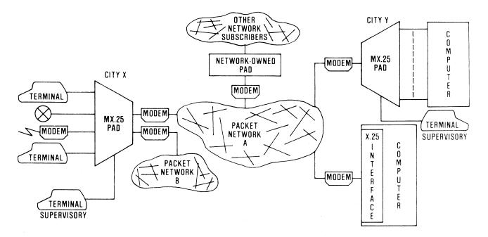
Figure 2. Typical Microplexer network application. If the unit is equipped with dual synchronous links, it can access more than one public data network.
