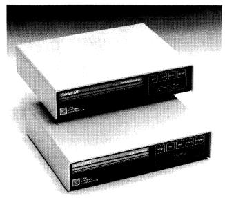
KMW's Series III protocol converters have been designed especially for communications applications requiring only one port. Presently, the Series III product line consists of the Twinax and Coax models.
