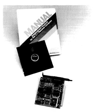
All of the AST communications products include an adapter card that fits into a single IBM PC expansion slot, software diskette, and documentation. The AST-5251, above, allows an IBM PC to emulate an IBM 5251 display terminal, for interactive communications with an IBM System/34, System/36 or System/38 computer system.
