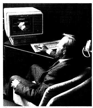
The newest addition to the Sperry UTS 4000 family is the UTS 60, a programmable terminal with color graphics capability. The UTS 60 features a 14½-inch display that features 16-color capability in graphics mode, and 8-color capability in alphanumeric mode. In addition to the terminal's standard Uniscope operating mode, the CP/M operating system is available for personal computer operation.
