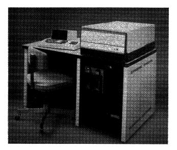
At the top of the Series 1500 product line is the Model 1503 Disc Processor. It is designed to provide multiple 1501 or 1502 Workstations with shared access to data files as large as 20 million characters.
