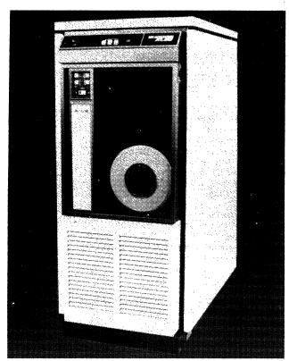
The XL50 is available in two models and can be configured with up to 32 terminals. Maximum system memory for both models is 512K bytes.
