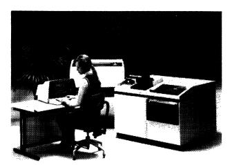
The Pertec XI.40 is a disk-based system that can support both local and remote keystations.
