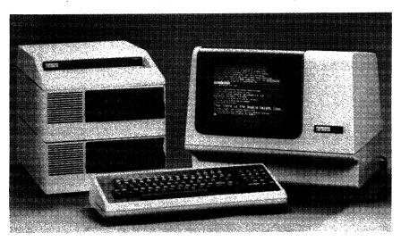
The PDT 11-150 shown here with dual diskette drives on the left is the top of the line of Digital Equipment's user-programmable terminal family. All models employ the LSI-11 micro-processor, making them fully compatible with the DEC PDP-11 minicomputer series.
