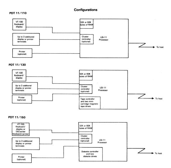
diskettes accommodated are single sided, IBM 3740 compatible, 8-inch diameter removable platters, each of which contains 77 tracks and stores 256K bytes for a total of 512K bytes of diskette storage.
