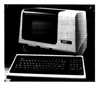
The PDT-11/130 consists of a VT-100 CRT, keyboard, and twin minicartridge tape drives, which are located in the base of the display and provide the system with 512K bytes of mass storage. Like the other PDT-11 models, the 130 employs an LSI-11 processor, making it fully compatible with the DEC PDP-11 minicomputer series.
