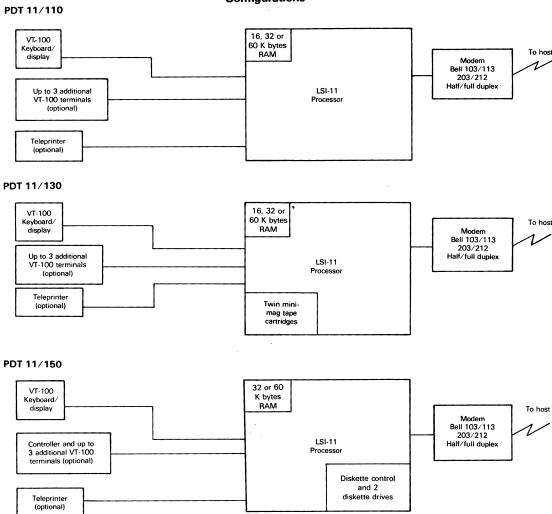
patible, 8-inch diameter removable platters, each of which contains 77 tracks and stores 256K bytes for a total of 512K bytes of diskette storage.
