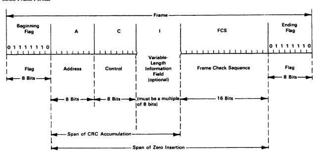
The transmission frame consists of Flag-Address-control-information-Frame Check Sequence-Flag. Each field has either eight bits or a multiple of eight bits.
