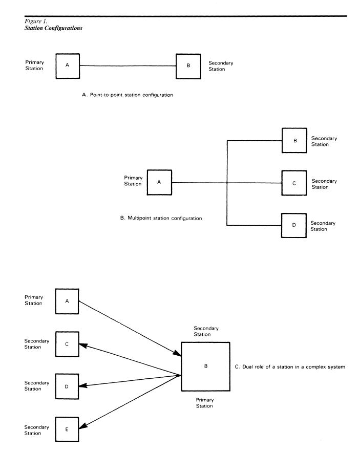
Besides the basic point-to-point or multipoint configurations, SDLC allows for configuration variations including half or full duplex and switched or nonswitched configurations.
