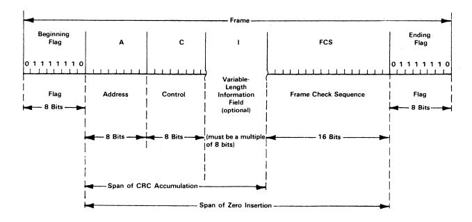
The transmission frame consists of Flag-Address-control-information-Frame Check Sequence-Flag. Each field has either eight bits or a multiple of eight bits.
