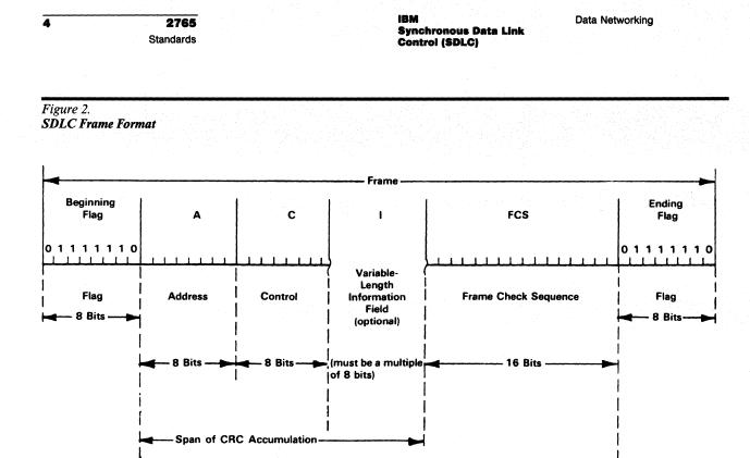
The transmission frame consists of Flag-Address-control-information-Frame Check Sequence-Flag. Each field has either eight bits or a multiple of eight bits.
