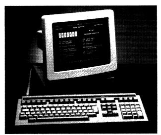
The WY-85 is Wyse Technology's DEC VT220 emulator. The terminal features ANSI X3.64 compatibility, a 14-inch tilt/swivel display with 80/132-column display capability, and a low-profile keyboard.
