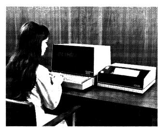
The Hazeltine 2000 is the most popular display terminal of the five models offered by the company. Included with the terminal shown above is the optional 30 cps thermal printer. The Hazeltine 2000 is marketed as a direct replacement for Teletype Model 33 and 35 units.
