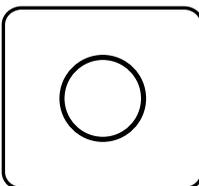
**POWER OFF:** This symbol indicates the principle on/off switch is in the off position.
