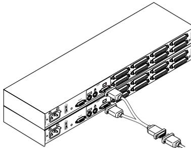
3. Connect the female VGA cable to the end of your monitor cable.
