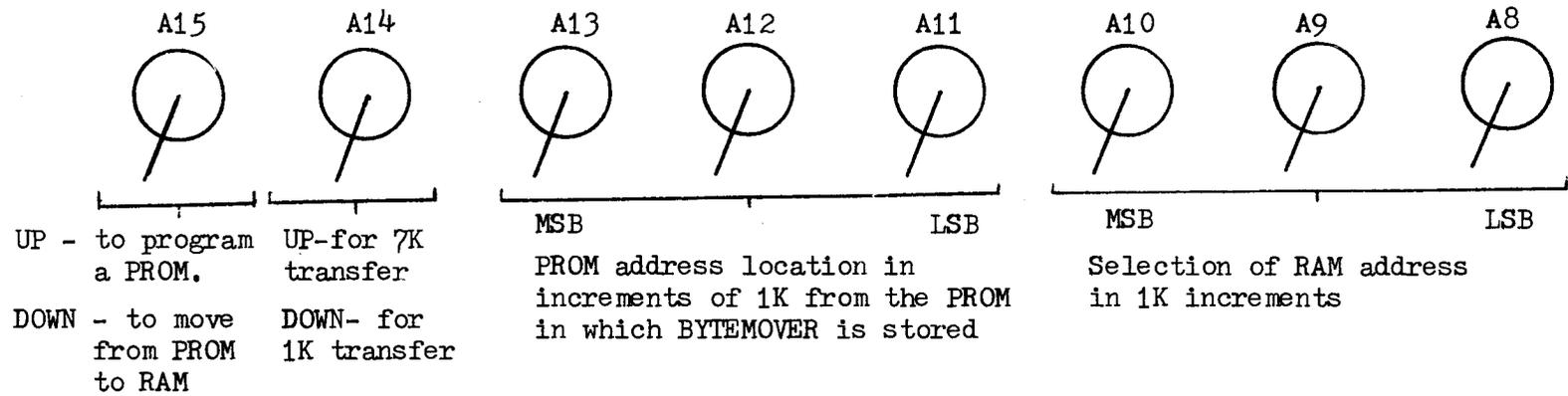
FIGURE 2. FUNCTION OF THE SENSE SWITCHES IN THE BYTEMOVER PROGRAM.
