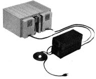
4 Plug a long line cord into the bottom connector at the back of the power supply.
