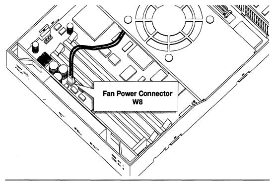
Figure 1-7: Cooling Fan Power Connection
