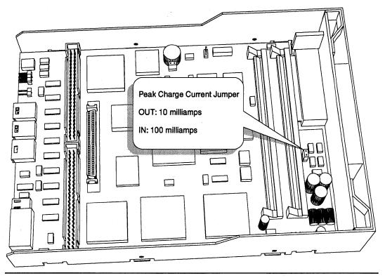
Figure 1-3: Peak charge current jumper
