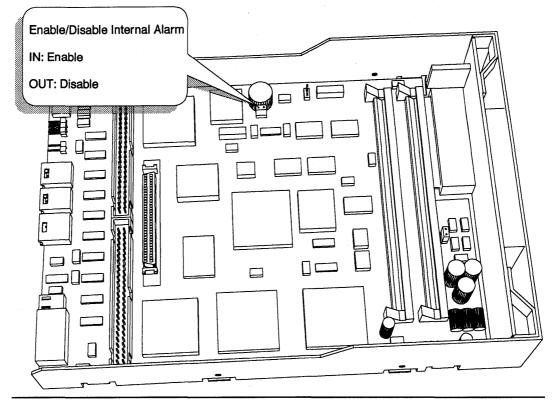
Figure 1-5: Enabling and disabling the internal alarm
