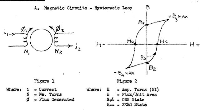
When a current  $I_1$  flows through winding  $N_1$ , a flux  $\emptyset$  is generated. A plot of  $I_1$  vs.  $\emptyset_1$  will result in the hysteresis loop shows in Figure 2. A more general graph is obtained if the axis of the hysteresis loop is changed from  $\emptyset$  to B, (B =  $\emptyset/A$ ) and I to H, (H = NI), generally referred to as the B-H curve, where B is flux density and H is the magnetizing force.
