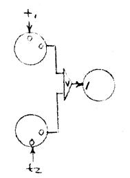
Same as above with both cores read out at different times. Designs are identical and one input winding is used.
