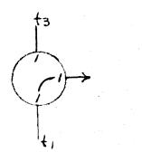
A core producing conditional transfer at time t1 when switched from the ZERO to the ONE state.
