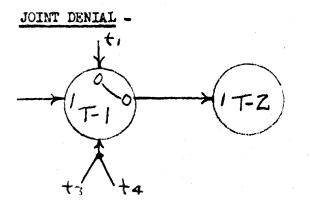
After T-1 is set to the ONE state a  $t_1$  input will transfer the ONE to T-2 unless  $t_3$  or  $t_4$  or both occur first which would kill the ONE in T-1.
