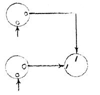
Two inputs of different designs ORed on separate windings.
