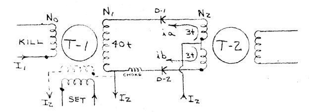
FIGURE 4 - BIASED DIODE OR SPLIT WINDING TRANSFER LOOP
