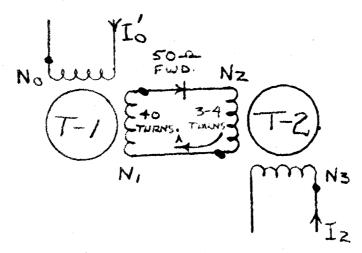
FIGURE 2 - SINGLE DIODE TRANSFER LOOP
