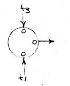
A core producing transfer if switched from the OME to the ZERO state at times  $t_1$  or  $t_3$ . This is unconditional transfer.
