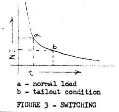
driver current thus taking switching current away from T-1. Due to the NI to Switching-Time relationship (FIGURE 3) <u>TAILOUT</u> will result. (Less Ampere Turns -More Switching Time required). The circuit is thus designed to allow for the extra tie to complete the switching of T-1.
