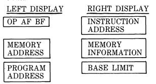
Each group is appropriately identified by a legend which is illuminated only when the numeric tube display is operating in that particular mode.
