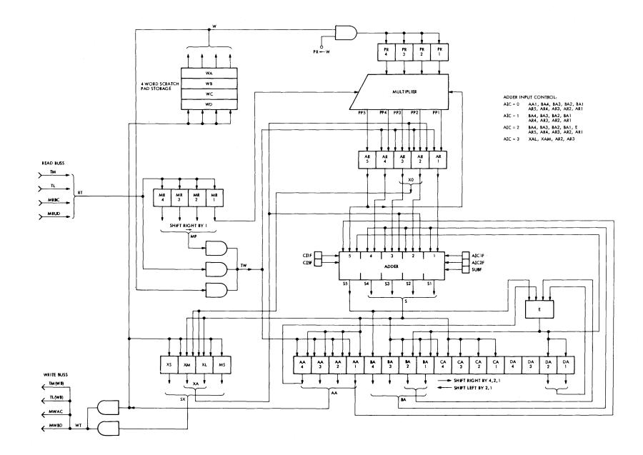
Figure 6. Fixed Length Arithmetic Unit
