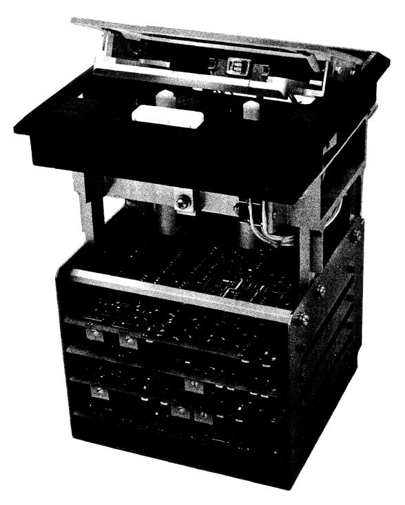
Reading a tape is accomplished at 10 inches per second in either the forward or the reverse direction. Writing is accomplished at 10 inches per second in the forward direction only. Data is written serially in the NRZI format at densities up to 800 bits per inch using two channels, one for data and the other for a synchronous clock.
