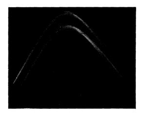
Figure 4-6. Read Skew Adjustment
