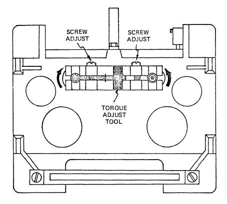
Figure 4-3. Brake Adjustment
