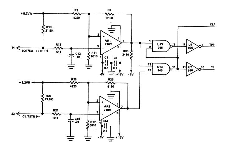
Figure 2-4. Dual Light Pipe Sensing Circuit
