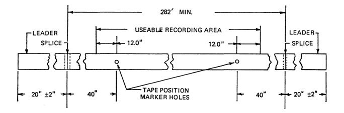
Figure 2-2. Tape Dimensional Requirements
