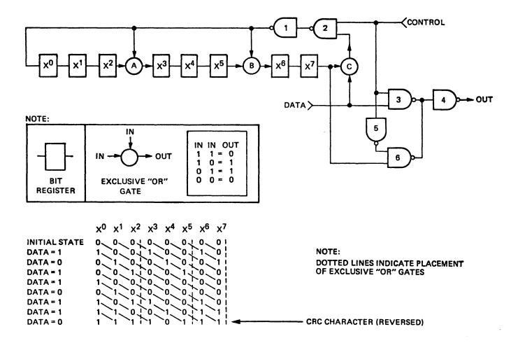
Figure 2-12. Typical CRC Register and Bit Shift Flow
