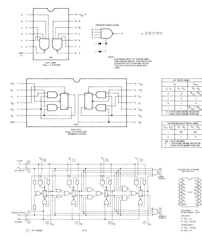
Figure 5-5. Chips and Special Components (sheet 2)
