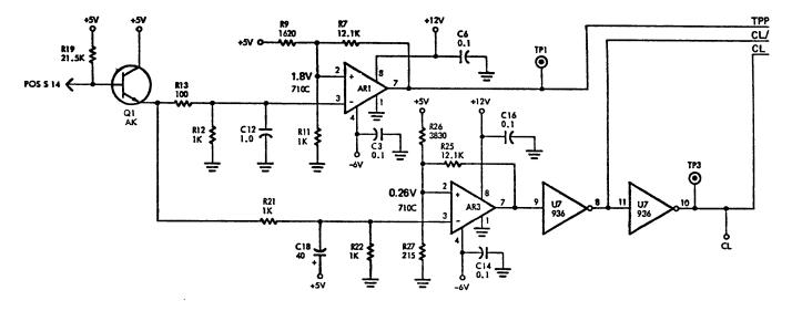
Figure 2-3. Single Light Pipe Sensing Circuit
