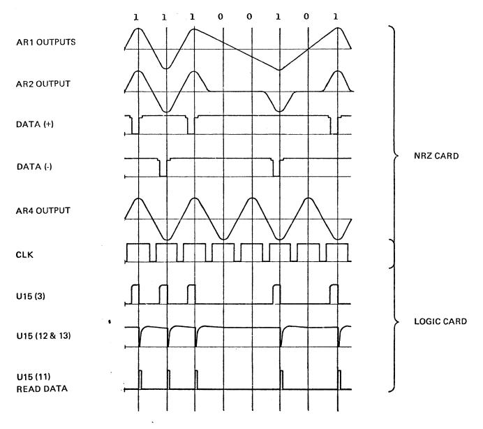
Figure 2-9. Read Data and Clock Levels
