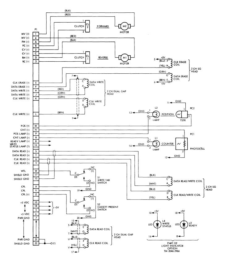
Figure 2-10. Deck Wiring (Single Light Pipe)
