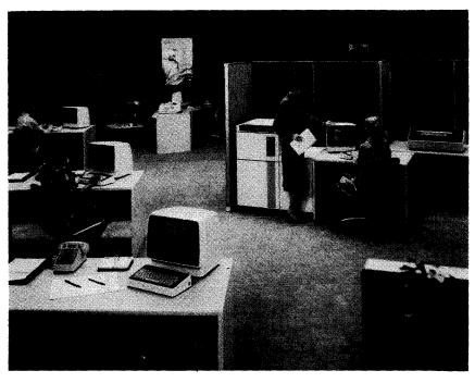
The B 930, available in Models 1 and 2, employs a multiple processor architecture. The system can employ up to eight processors, each with an associated memory module. The B 930, which operates in Burroughs' Computer Management System (CMS) software environment, supports up to 3.2MB of main memory, 1.7GB of online disk storage, and 36 concurrently active workstations.
