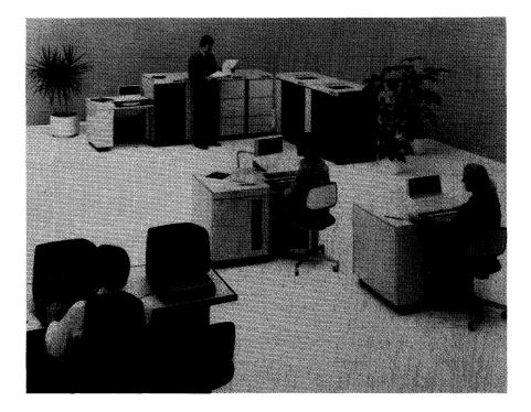
This large configuration of the Burroughs B 820 system covers most of the bases. In the foreground are two TD 830 CRTs at left, a Direct Data Entry Station (DDES) at right, and an AE 500 Audit Entry Station with two Super Mini-Disk drives in the center. From left to right in the back-ground are the DDES console, a double-width B 820 processor, two disk pack drive cabinets, and two line printers.
