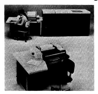
Burroughs' new AE 301 Audit Entry Computer (foreground) can be used as an off-line data entry station to prepare cassette tape for entry into the B 700 computer system shown in the background. From left to right are the B 700 console with cassette tape subsystem, processor, dual disk cartridge drive, and line printer.
