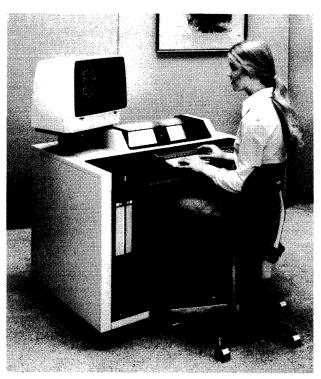
The B 91S is a console-based system for general business data processing. It has 256KB of main memory and includes a 230-cps console printer with keyboard. The B 91S can be expanded to support 512KB of memory, 154MB of disk storage, and eight workstations.
