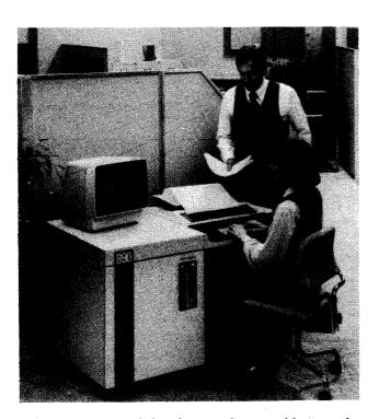
The B 92 is a console-based system for general business data processing. It has 256KB of main memory and includes a 120 cps console printer with keyboard. The B 92 can be expanded to support 512KB of memory, 154MB of disk storage, and eight workstations.
