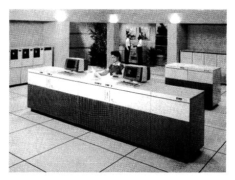
The Burroughs A 10 H is an intermediate-range, dual-processor mainframe with up to 96 megabytes of main memory, two I/O cabinets with a maximum of 80 DLPs, and up to 288 data communication lines. main memory, but has no cache memory. The multiply/ divide accelerator feature, which enhances the performance in applications involving repetitive operations using the multiply and divide functions, is only available on the A 10F and A 10 H and not on the A 10 D.
