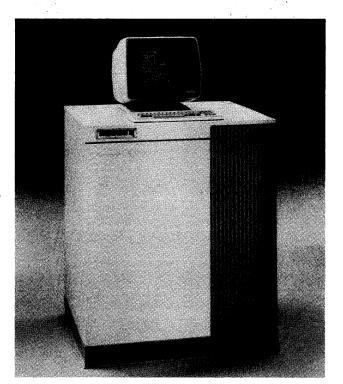
The Burroughs' A 5 Model F has a main memory range of 6 to 24 megabytes, and supports up to 16 Data Link Processors.
