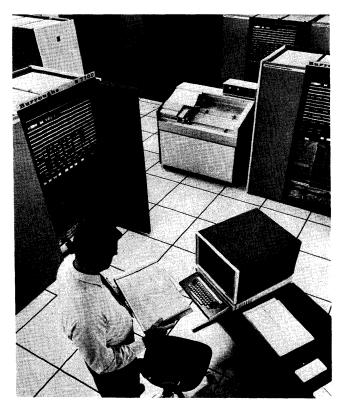
The B 7700 is the largest and most advanced computer in Burroughs' broad "700 Systems" product line. The B 7700 central exchange can accommodate up to 6 million bytes of core storage and a total of up to 8 central processors and input/output processors.
