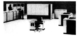
The one announced model in the B 3900 series of the Burroughs 900 family is the B 3950. As a companion to the smaller B 2930, the B 3950 offers greater expandability with up to five million bytes of main memory and up to 32 data link processors. As with the B 2930, up to four B 3950 Central Processors can be interconnected to form a multiprocessor system.
