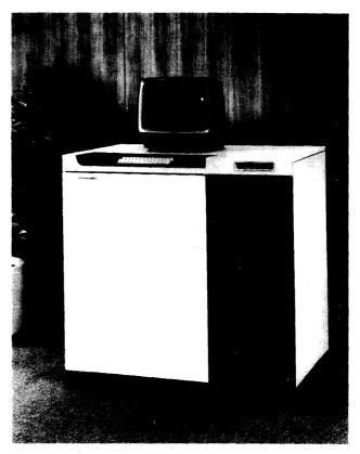
Burroughs claims the newer B 1800 processors offer significant price performance improvements over the older models. The B 1815, B 1855, and B 1885, which now make up the actively marketed B 1800 product line, occupy 50 percent less floor space and consume 25 percent less electrical power than the older processor models such as the B 1870.
