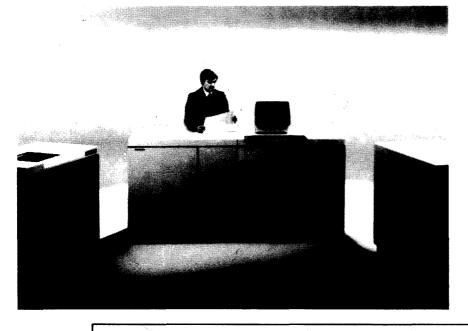
Burroughs claims the B 1885, shown here, is the first system in its price class to offer two independent central processors. The processors share the main memory, which can extend from 512K bytes to 1.02 megabytes. One processor acts as a slave in this configuration, with the MCP operating system residing only in the master processor.
