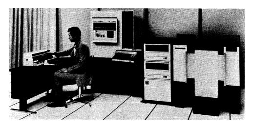
This basic B 1700 configuration consists of (from left): 96-column card reader/punch equipped for off-line use as a data recorder, central processor with console printer, dual disk cartridge drive, and line printer.
