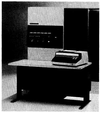
The B 1700 Series console has recently been restyled as shown above. It is functionally the same as the earlier console design shown in the preceding photos.
