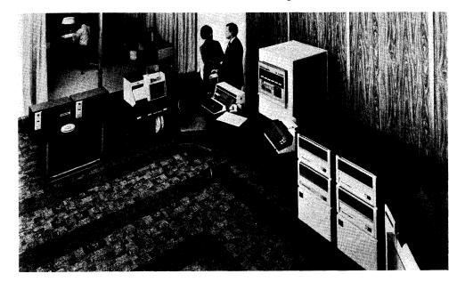
This medium-sized B 1700 System is equipped with two of Burroughs low-cost 10KB magnetic tape drives (far left) and a pair of dual disk cartridge drives.
