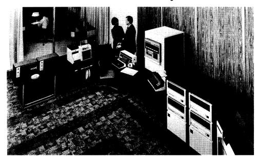
This medium-sized B 1700 System is equipped with two of Burroughs' new, low-cost 10KB magnetic tape drives (far left) and a pair of dual disk cartridge drives.
