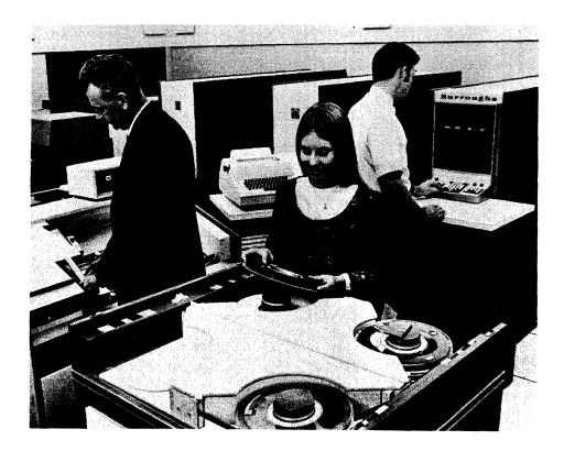
This B 3500 installation at W i s c o n s i n S t a t e University-Eau Claire includes a three-drive Magnetic Tape Cluster (foreground) and a 1400-cpm card reader (at left). The central processor and console are at right.
