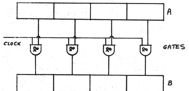
Figure 4. Example of register enable using AND gates.
