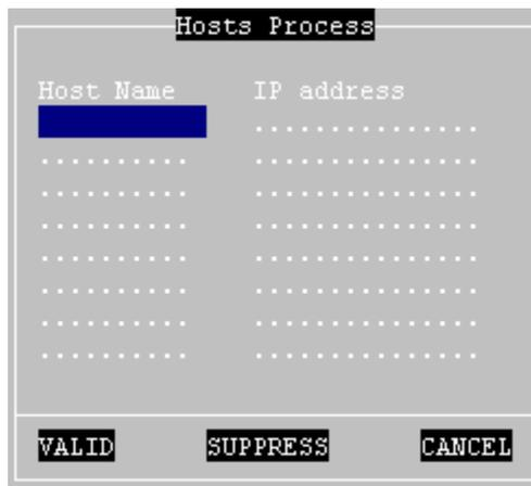
**Add a Host:** move the highlight cursor to a vacant line and enter the name and IP address of the host.
