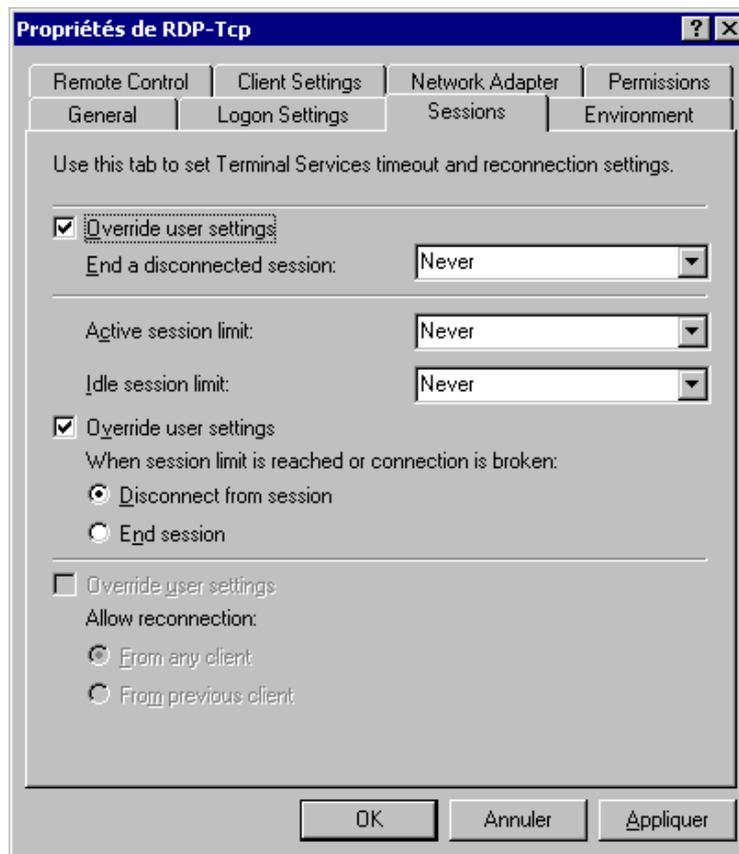
Enable the 'Override user settings' check box and set the required delay for the 'Idle session limit' parameter.
