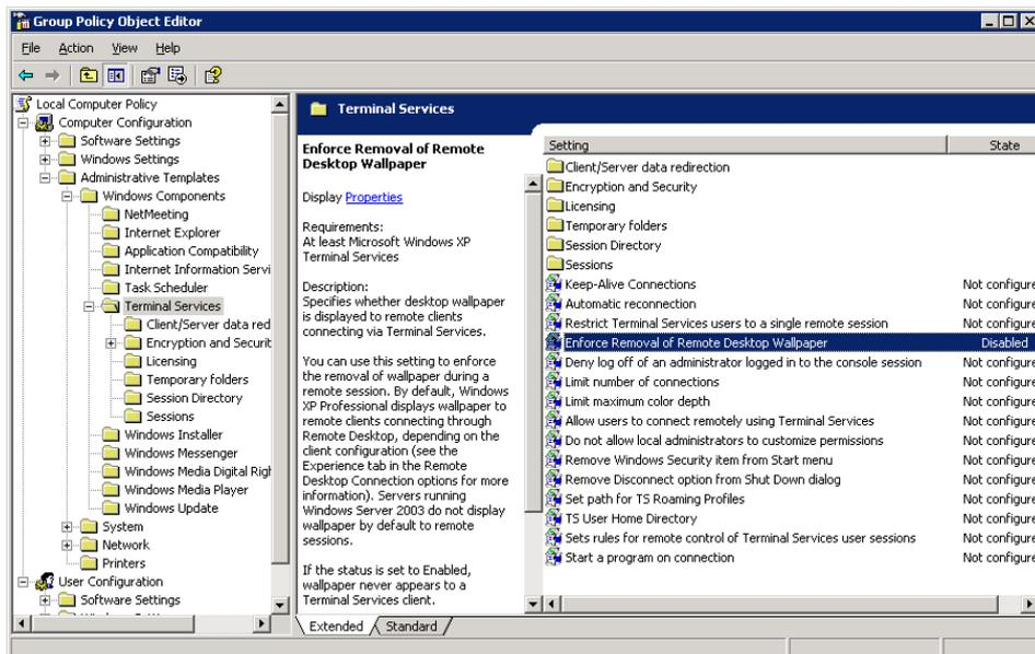
Expand the tree to [Computer Configuration]-[Administrative Templates]-[Windows Components]-[Terminal Services]. Set the parameter "Enforce Removal of Remote Desktop Wallpaper" to "Disabled".
