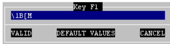
The main field is used to enter the programmable key value. ASCII codes lower than 20h can be entered as '\xx' (where xx is the hexadecimal value of the ASCII code).
