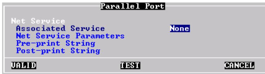
The **[TEST]** button allows communication between the AX3000 auxiliary port and the parallel device to be tested. Whatever the auxiliary port status (TCP/IP connection established or not), when this button is 'pressed', data is sent from the AX3000 port to the device.
