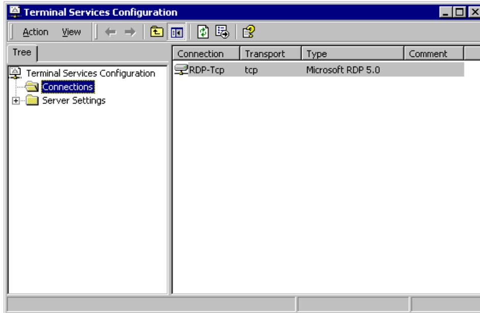
To configure the RDP server, select 'Connections' in the left panel, then double-click the line 'RDP-Tcp' on the right panel. Another dialog box is displayed. It allows setting:
