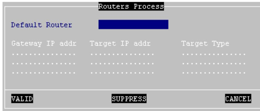
**Default Router:** to specify a default router, enter its IP address. If a default router is not required, leave this field blank
