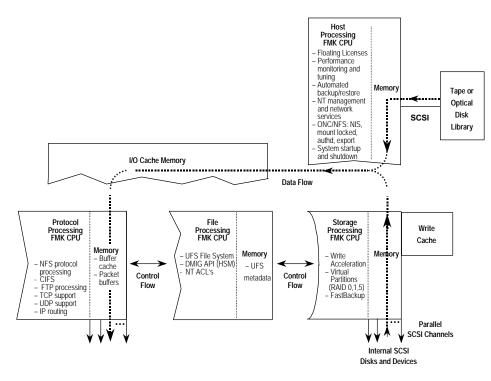
Figure 10: The NetServer functional multiprocessing I/O architecture. All protocol, file system, and storage processing is completely removed from the UNIX host processor. The UNIX host processor, a SPARC-based design, is responsible for system booting, ONC functions, error logging and reporting, performance monitoring, SNMP agent coordination, backup and restore, and virtual partition and file system cloning administration.
