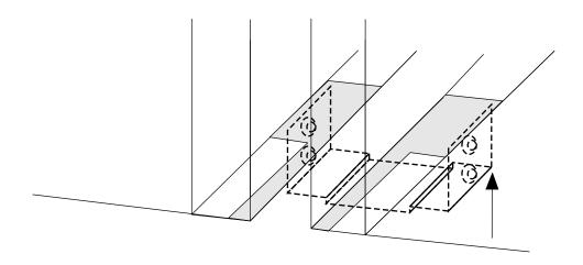
Figure 3-3. Lining up the U-shaped bracket
