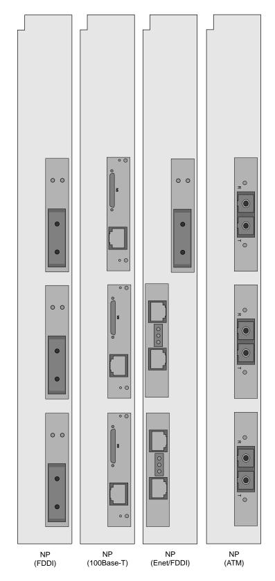
Figure 3-15. Location of network ports on mixed NP boards
