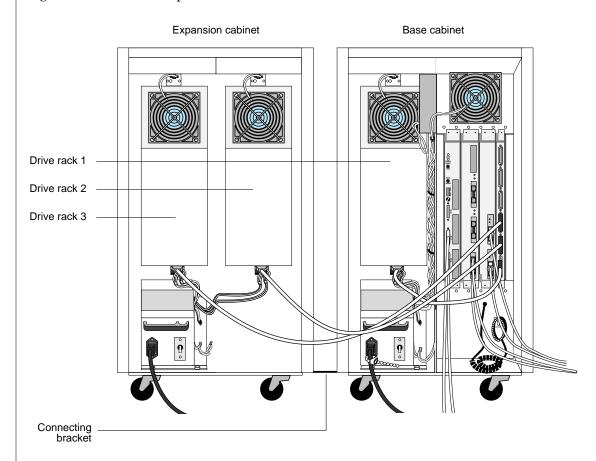
Figure 3-6. Back view of connected cabinets
