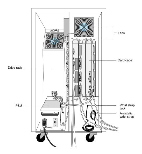
Figure 2-4. Base cabinet subassemblies (back view)
