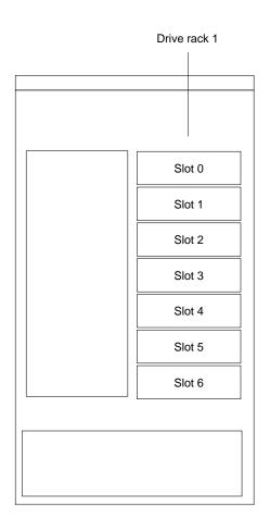
Figure 3-17. Base cabinet drive slot numbering
