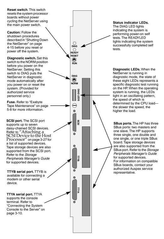
Figure 2-7. HP front panel connectors
