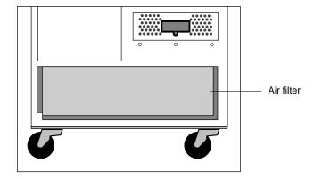
Figure 5-1. Air Filter location (front view of base cabinet)
