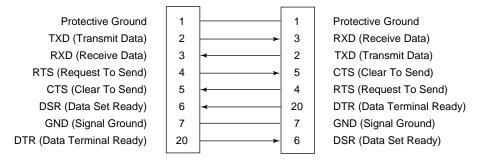
Figure B-1. Console cable pin diagram
