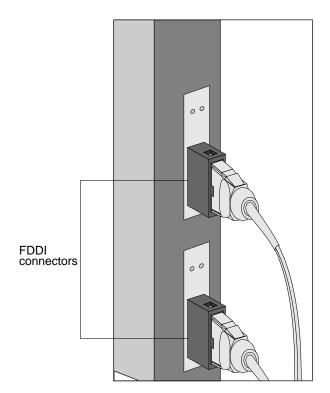
Figure 3-11. Connection to FDDI (fiber) ports
