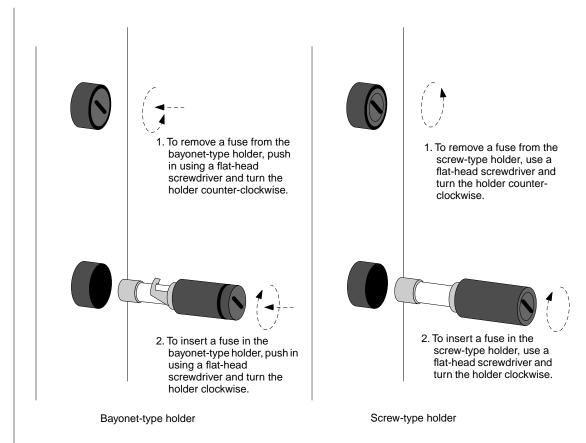
Figure 5-2. HP fuse holder types
