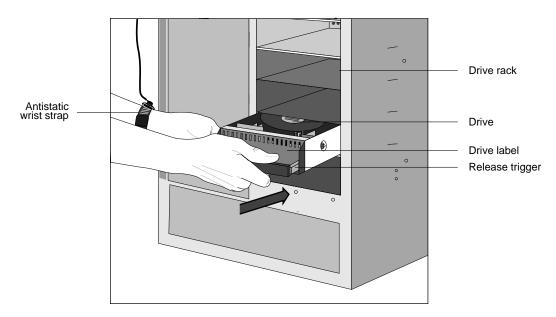
Figure 3-20. Installing a drive
