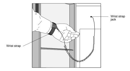
Figure 3-2. Antistatic wrist strap
