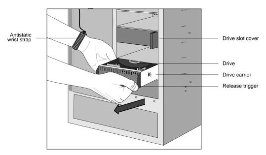
Figure A-4. Removing a drive
