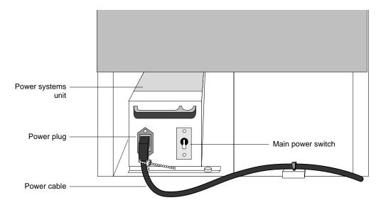
Figure 3-1. Main power switch (back view of NetServer)
