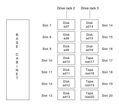
Figure A-2. First expansion cabinet with fourteen drives (front)
