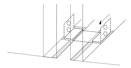
Figure 3-4. Installing the U-shaped bracket
