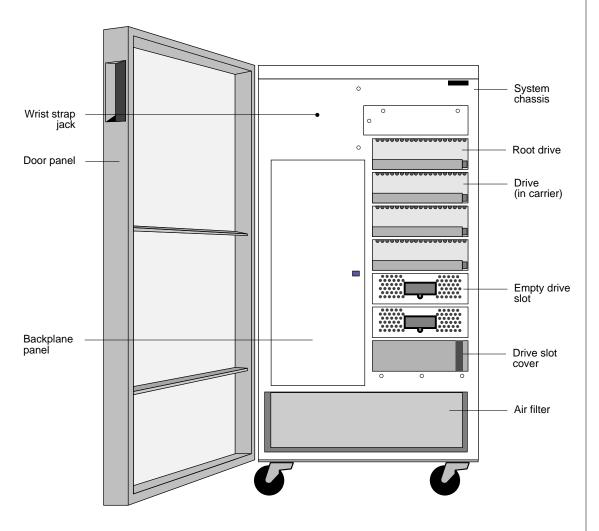
Figure 2-3. Base cabinet subassemblies (front view)
