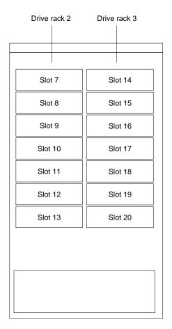
Figure 3-18. First expansion cabinet drive slot numbering
