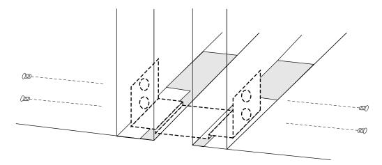
Figure 3-5. Attaching the U-shaped bracket
