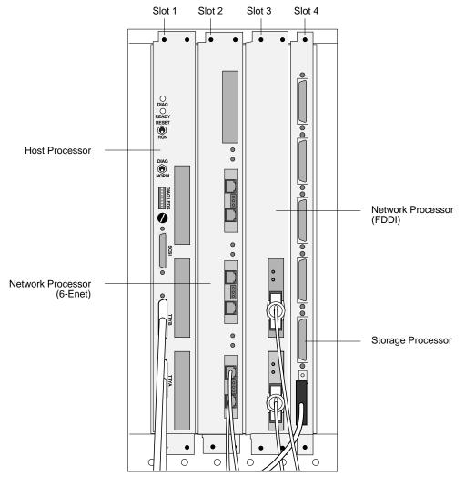
Figure 2-8. System processors
