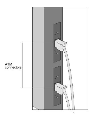
Figure 3-14. Connection to ATM (UTP) ports
