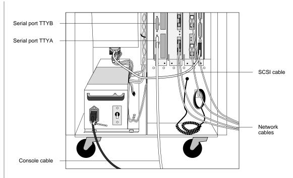
Figure 3-7. Routing cables to the NetServer
