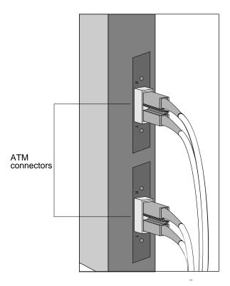
Figure 3-13. Connection to ATM (fiber) ports
