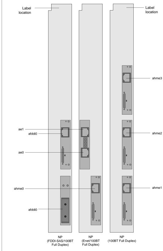
Figure 3-16. Example of network interface numbering
