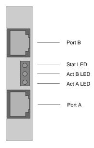
Figure 4-2. 10Base-T Ethernet LED display
