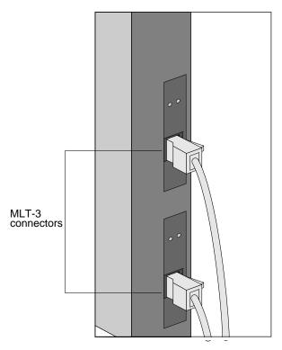
Figure 3-12. Connection to FDDI (MLT-3) ports
