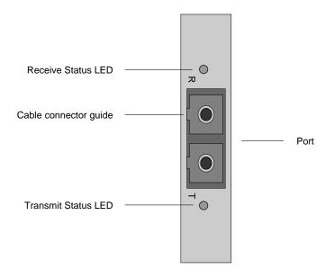
Figure 4-1. ATM (fiber) LED display
