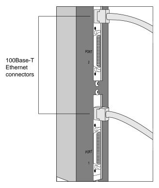
Figure 3-10. Connection to 100Base-T (full duplex) ports
