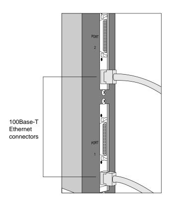
Figure 3-9. Connection to 100Base-T (half duplex) Ethernet ports
