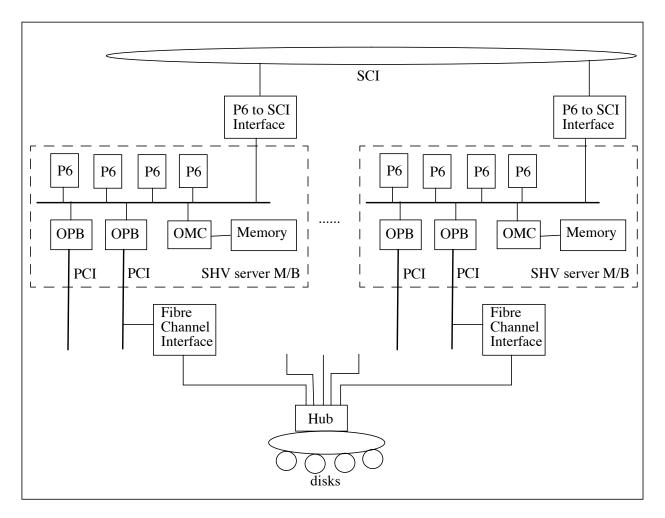
This is a true SMP architecture. They are connecting Standard High Volume (SHV) 4 way P6 motherboards from Intel together on SCI and implementing the directory based coherency protocol designed as the IEEE SCI standard. Like Sun, they are going to take advantage of Fibre Channel disk drives and switches to connect the disk storage.
