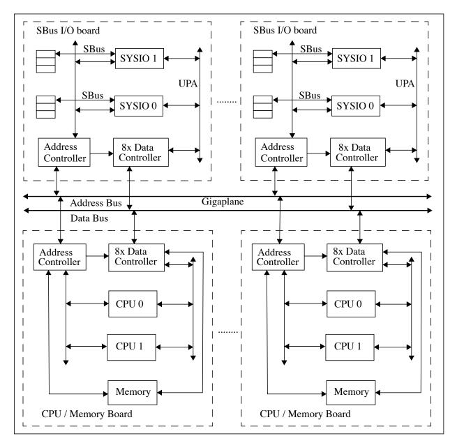
This is a fairly classic SMP kind of design. In order to be able to effectively support multiple processor boards, all using a snooping cache coherency protocol, a very fast system interconnect is required.
