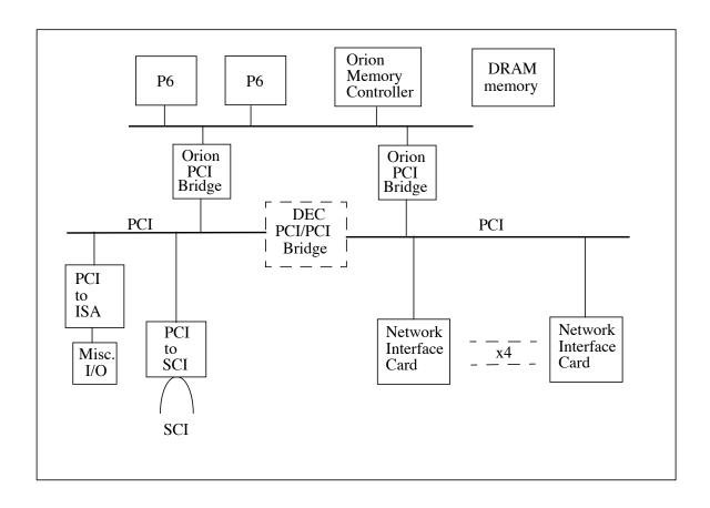
The DEC PCI/PCI bridge is in dotted lines because in the first implementation this bridge is unused. It is simply there because we are using the same motherboard as the FSP.
