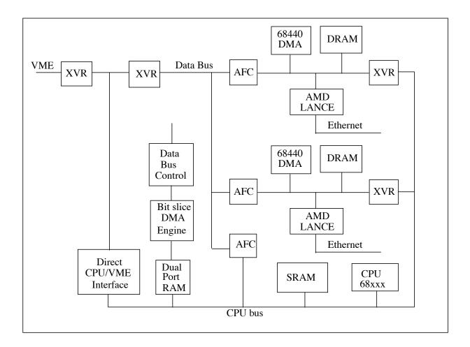
Again notice that the main data bus is separate from the CPU bus. Ethernet packets are stored in DRAM on the Ethernet bus. The headers in DRAM memory may be read by the processor, but all the actual data can be transferred via the VME bus without ever appearing on the CPU bus. The DRAM memories and the associated logic are duplicated for more performance.
