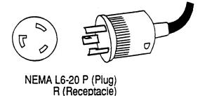
Figure 3-1 Power Plug Diagram
