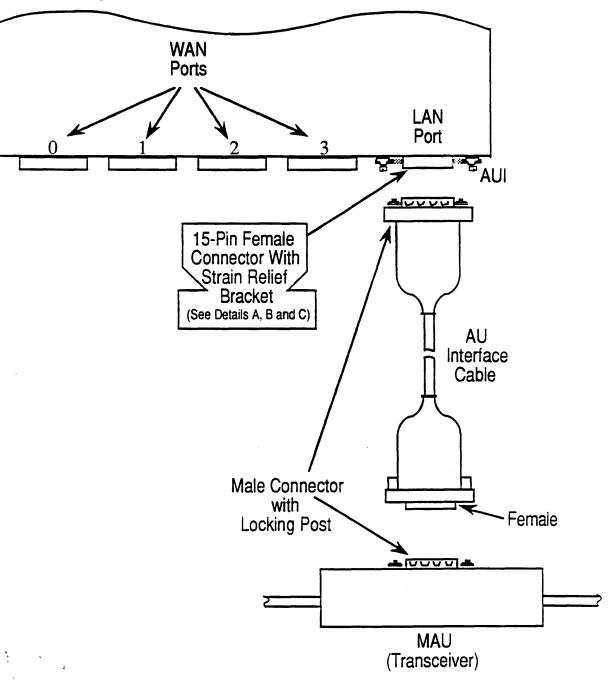
Figure B-2 Connector Hardware and AUI Cable Configuration
