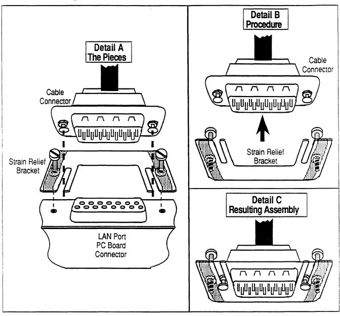
Figure B-3 LWDB Connector Hardware and AUI Cable Detail
