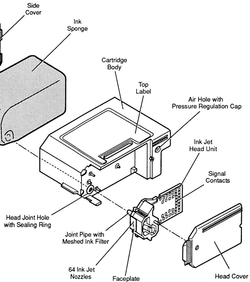
**Figure 1-2 Ink Cartridge Structure**
