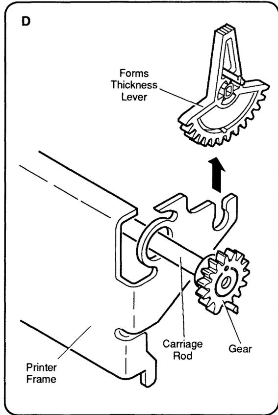
**Figure 2-7 Forms Thickness Lever**
