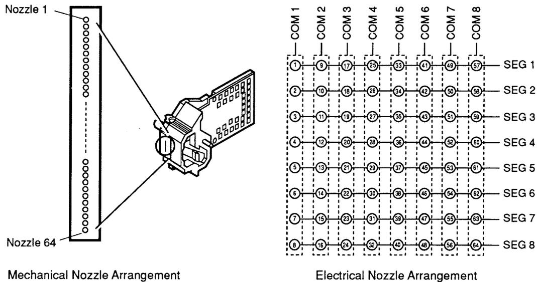
**Figure 1-4 Nozzle Arrangement**
