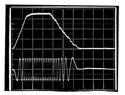
WAVEFORM: Velocity and Position A (Forward and Rev Seeks)
