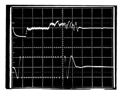
WAVEFORM: Current Sense and Position A (Forward and Reverse Seeks)
