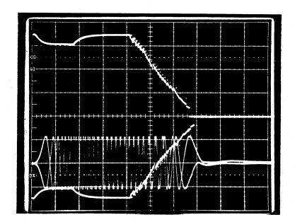
WAVEFORM: Curve Shift Function and Position A (Forward and Rev Seeks: 1 track)
