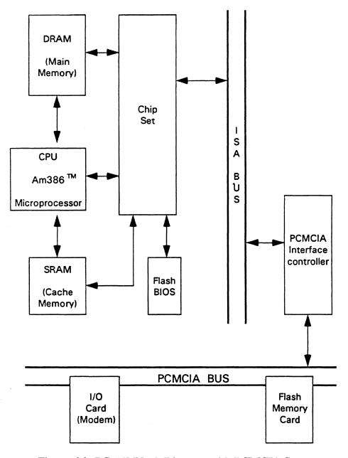
Figure 6.2 PC-AT Block Diagram with PCMCIA Support
