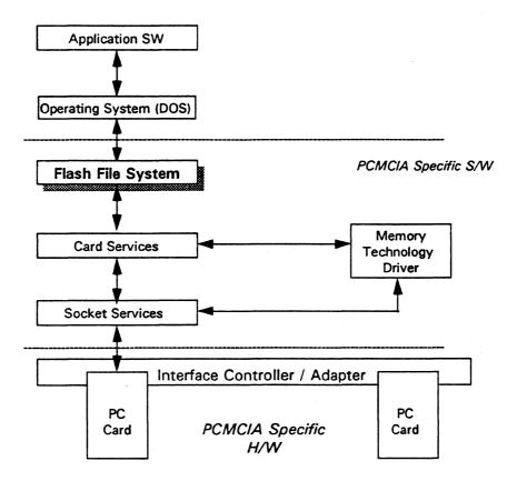
Figure 7.6 The PCMCIA Layers: Focus on the Flash File System
