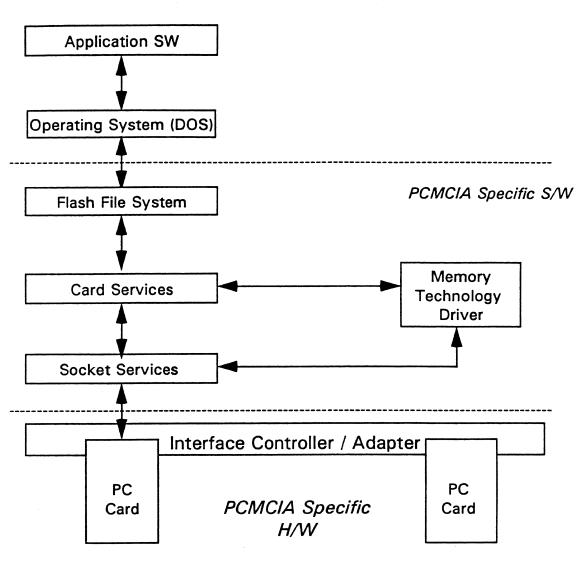
Figure 4.2 The PCMCIA Hardware and Software Layers
