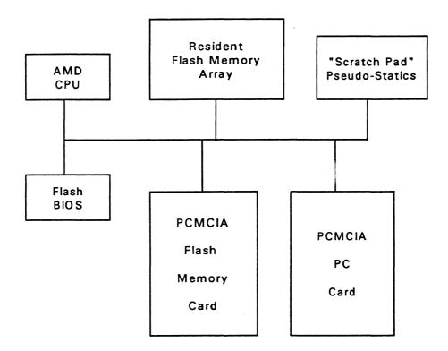
Figure 3.2 Emerging Memory Architecture
