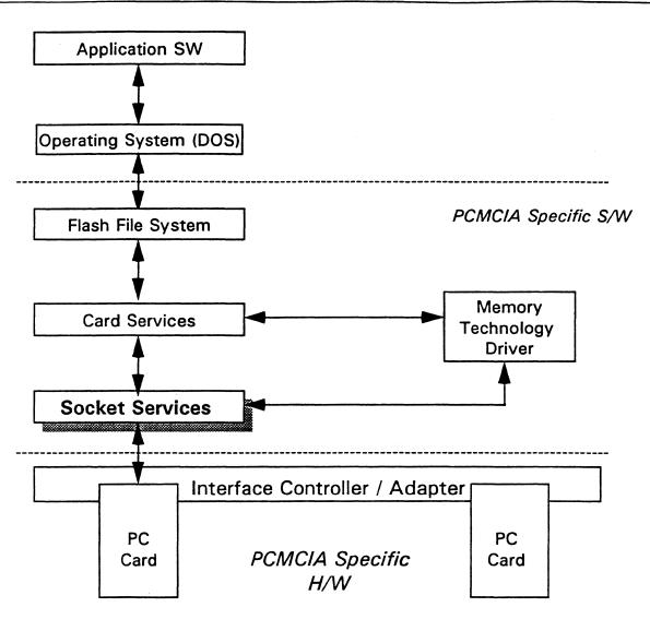
Figure 6.4 The PCMCIA Layers: Focus on Socket Services
