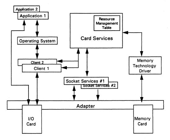
Figure 7.5 Card Services Software Architecture
