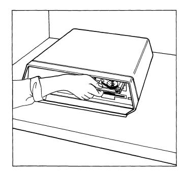
Figure 8. Inserting and Removing a Tape Cartridge
