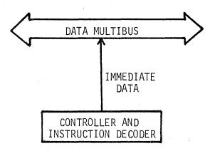
The instructions are often used to load registers in the various register files (i.e., the I and X Register Files in DEP, the Temporary Register File in ARP, and the General Register File in COP).
