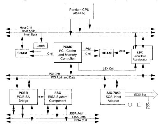
Interfacing the AIC-7850 to the Intel 82430 PCI Chipset (EISA Version)
