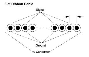
0.050-inch pitch, AWG28 PVC =  $100\Omega$ 0.050-inch pitch, AWG26 PVC =  $80\Omega$ 0.050-inch pitch, AWG30 PVC =  $80\Omega$
