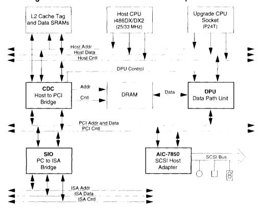
Interfacing the AIC-7850 to the Intel 82420 PCI Chipset
